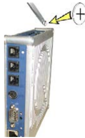
Fig. 45: Replacing the battery at the LCC
