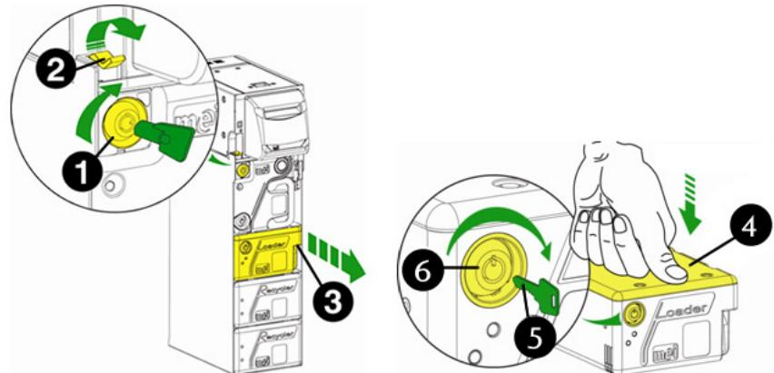
Fig. 102: Removing and opening the loader cassette
