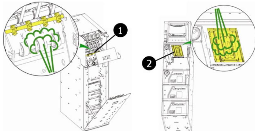
Fig. 111: Cleaning the test unit and the main module from the bottom
