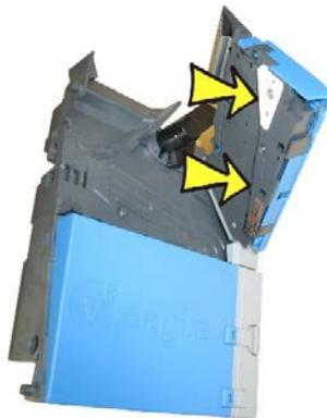
Fig. 79: Cleaning of the lower edge of the coin route
