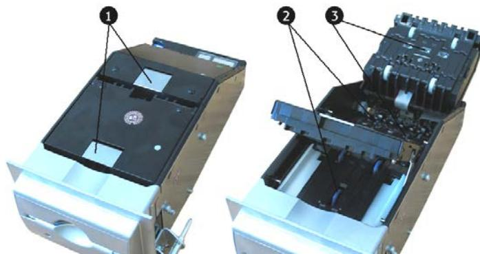
Fig. 89: Cleaning the banknote reader
