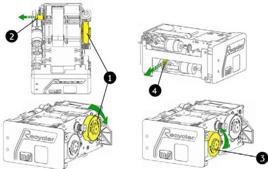
Fig. 115: Recycling cassette: Removing trapped banknotes
