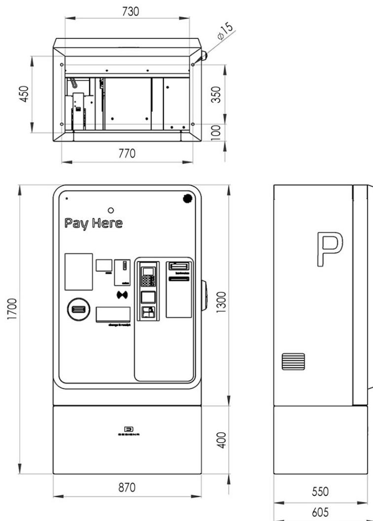
Fig. 5: Pay Cash&Card, with optional illuminated frame, dimensions in mm
