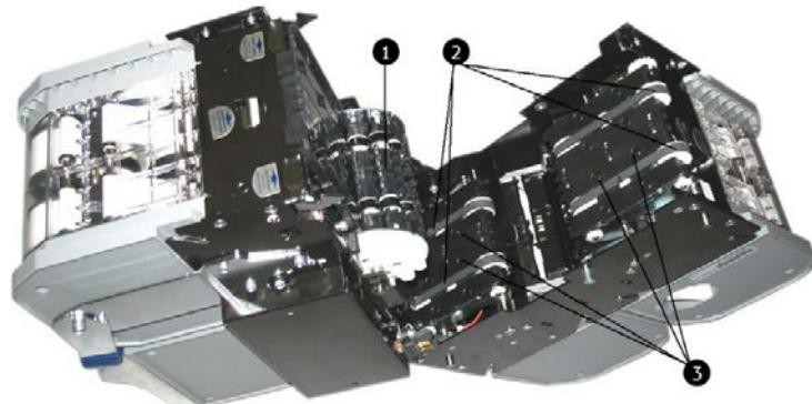
Fig. 92: Cleaning the chassis
