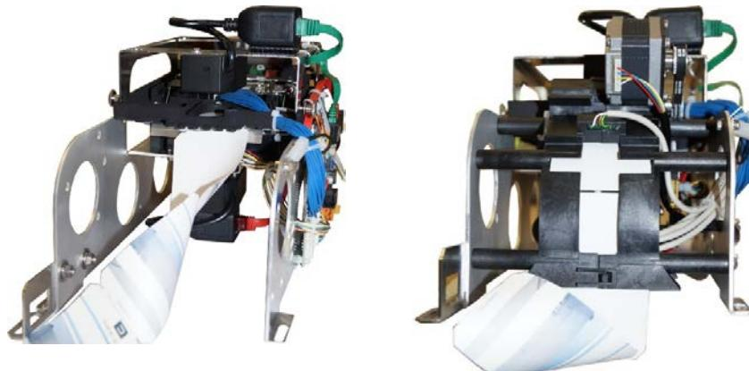
Fig. 68: Multicon MC Barcode: Without double feeding unit (left), with double feeding unit (right)
