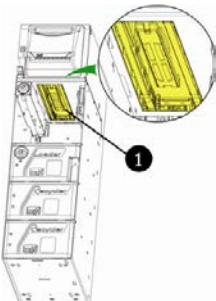
Fig. 113: Banknote cassette-pressure plate
