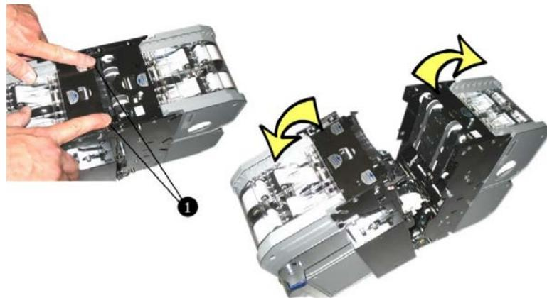
Fig. 91: Opening the chassis
