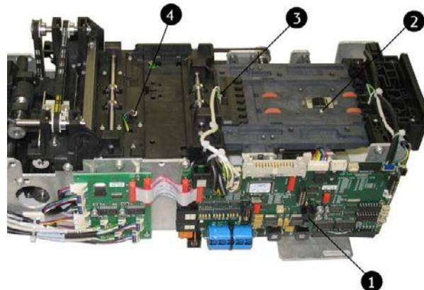
Fig. 60: Live LED and light barrier for error analysis
