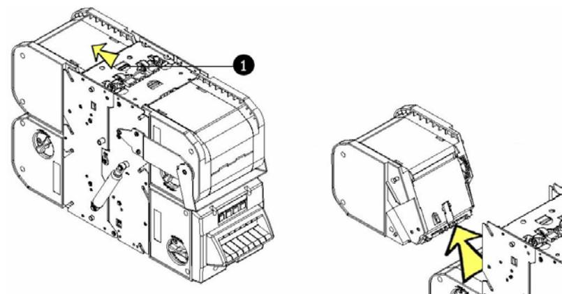
Fig. 94: Removing the recycling or (multi-)escrow cassettes
