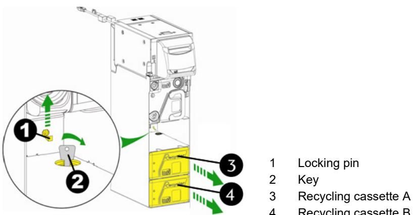
Fig. 114: Removing the recycling cassette
