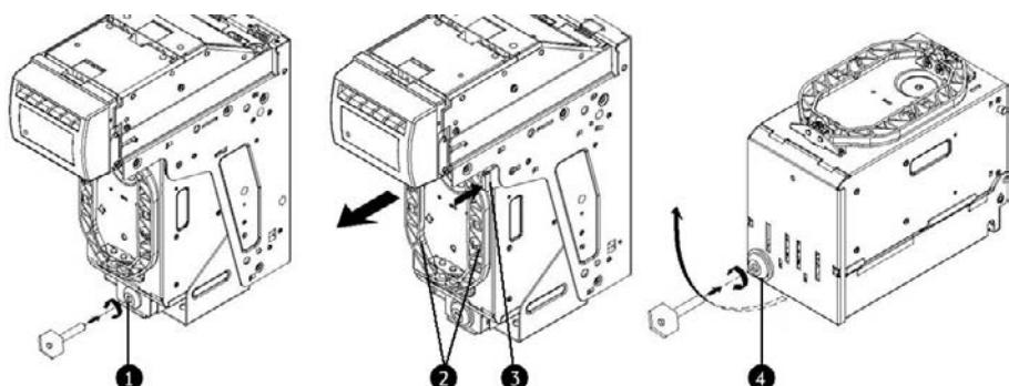
Fig. 84: Removing and opening the MFL stacker cassette (Figure with options)
