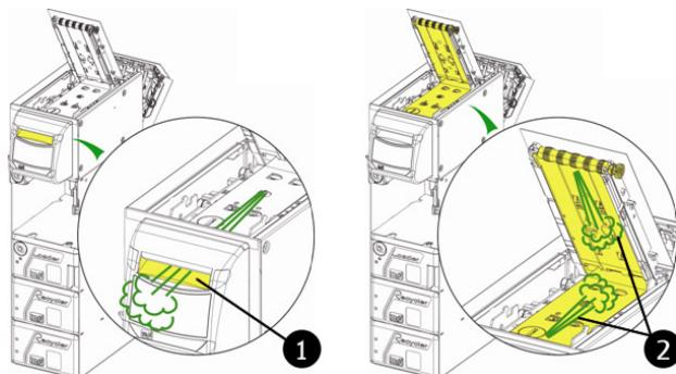
Fig. 108: Cleaning the banknote accepter and the positioner
