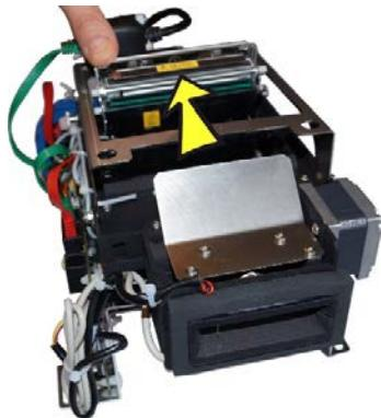
Fig. 69: Folding up the thermal line
