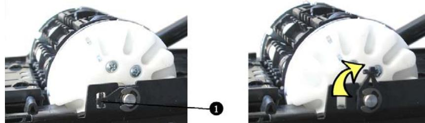
Fig. 93: Removing the path switch
