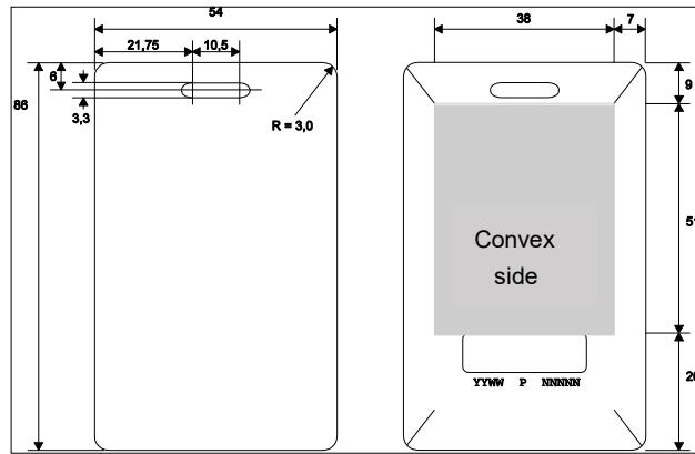
Fig. 117: EasyMove card (active): Approx. dimensions in mm
