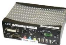
A *LAN box* is installed for the optional banknote recycler BNR MEI. This box is connected to the **TCC** via **Ethernet** and assumes communication with the banknote recycler via the USB interface.
