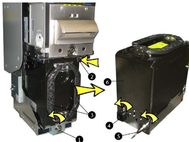
Fig. 87: Removing and opening the banknote cassette
