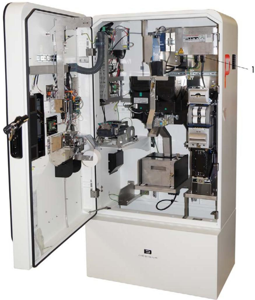
Fig. 39: Measuring point for measuring the fault loop impedance
