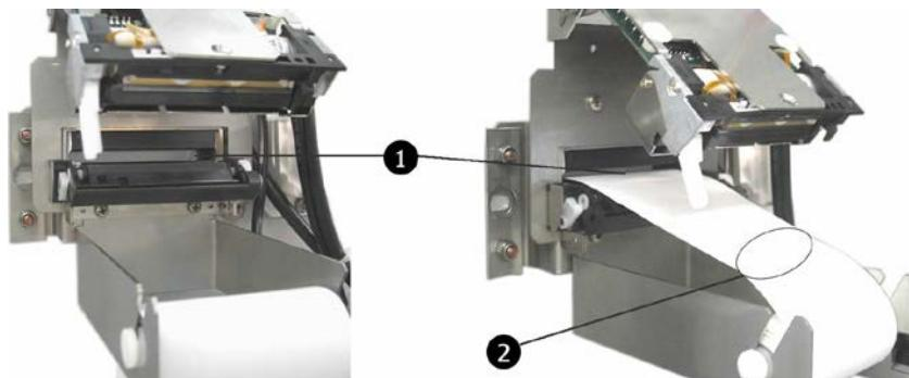
Fig. 73: Feeding paper into the draw-in device
