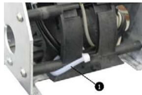
Fig. 48: Feeding channel I blocked
