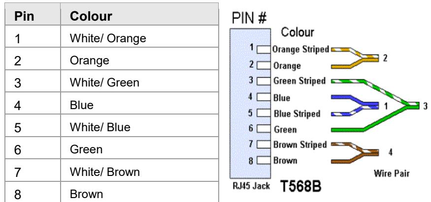
Fig. 36: Assignment of the Ethernet connection, EIA/TIA-T568B
