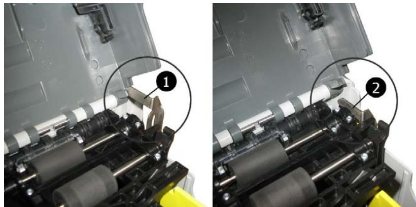
Fig. 103: Loader cassette, locking latch: correct position (left), wrong position (right)
