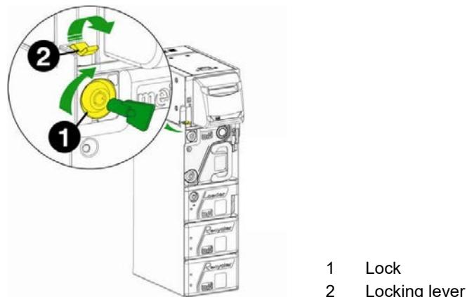
Fig. 100: Locking mechanism
