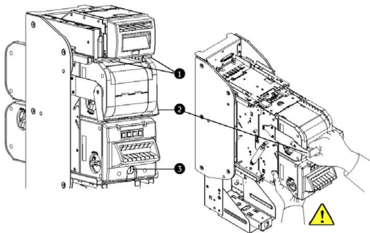
Fig. 90: Removing the chassis
