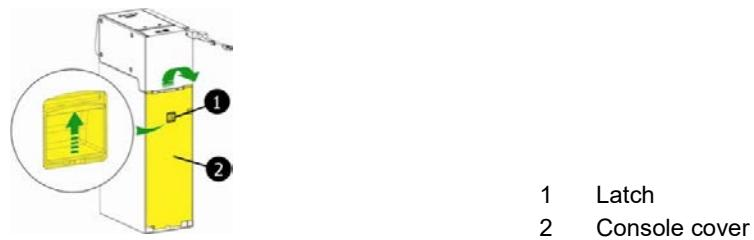
Fig. 110: Opening the console cover
