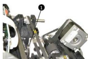
Fig. 50: Cuchilla autoafilable
