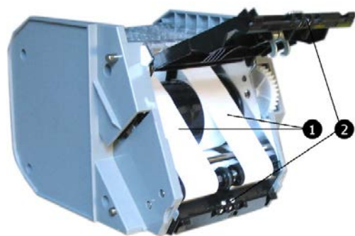
Fig. 92: Cleaning the recycling or (multi-)escrow cassettes
