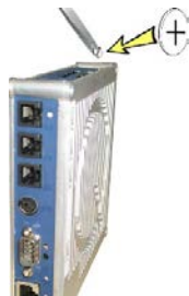
Fig. 39: Replacing the battery at the LCC
