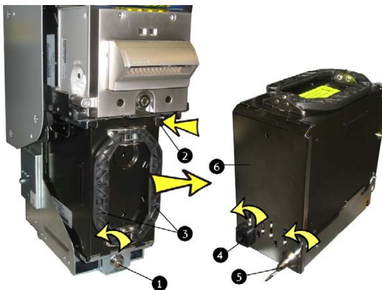
Fig. 83: Removing and opening the banknote cassette
