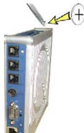
Fig. 39: Replacing the battery at the LCC
