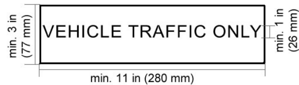
Fig. 3: Gate's danger zone sign II
