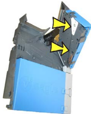
Fig. 75: Cleaning of the lower edge of the coin route
