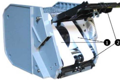
Fig. 92: Cleaning the recycling or (multi-)escrow cassettes
