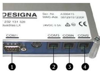
Fig. 40: Serial interfaces
