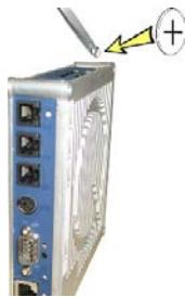
Fig. 42: Replacing the battery at the LCC
