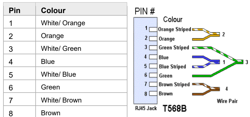
Fig. 37: Assignment of the Ethernet connection, EIA/TIA-T568B
