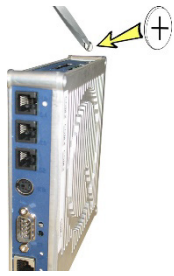
Fig. 45: Replacing the battery at the LCC
