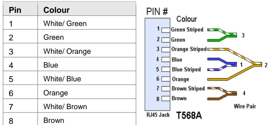
Fig. 35: Assignment of the Ethernet connection, EIA/TIA-T568A
