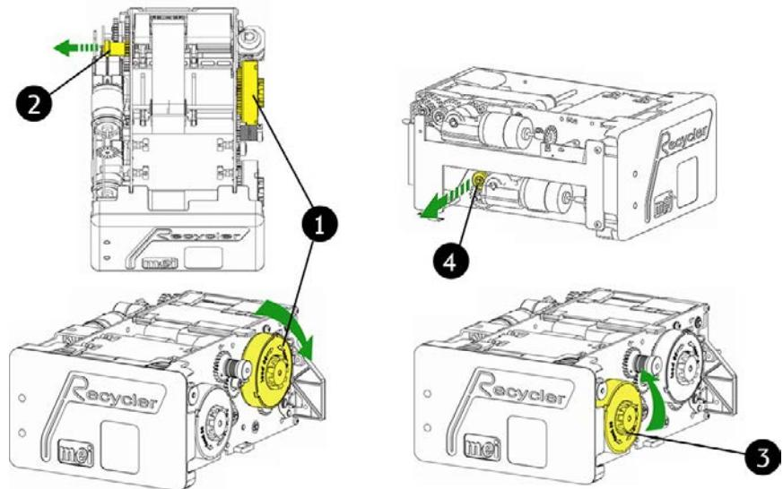
Fig. 104: Recycling cassette: Removing trapped banknotes
