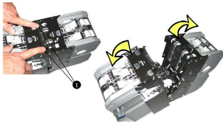
Fig. 80: Opening the chassis
