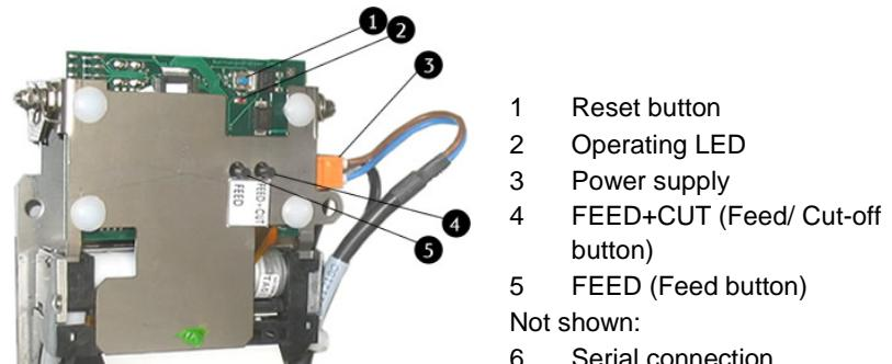
Fig. 72: PCB receipt printer
