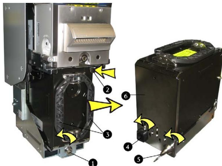
Fig. 76: Removing and opening the banknote cassette
