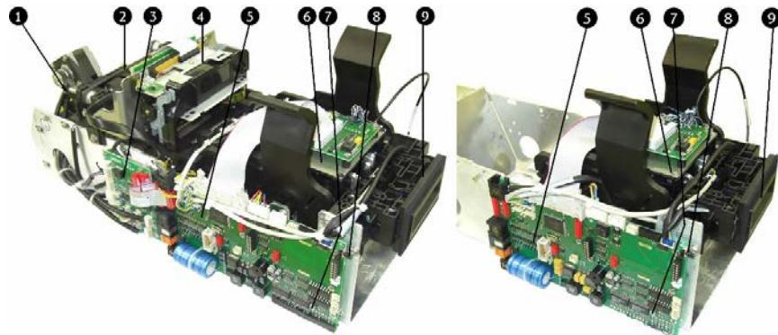
Fig. 46: Multicon with magnetic strip technology (example for equipment at ENT (left) and EXT (right))
