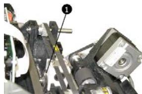
Fig. 50: Self-sharpening cutter
