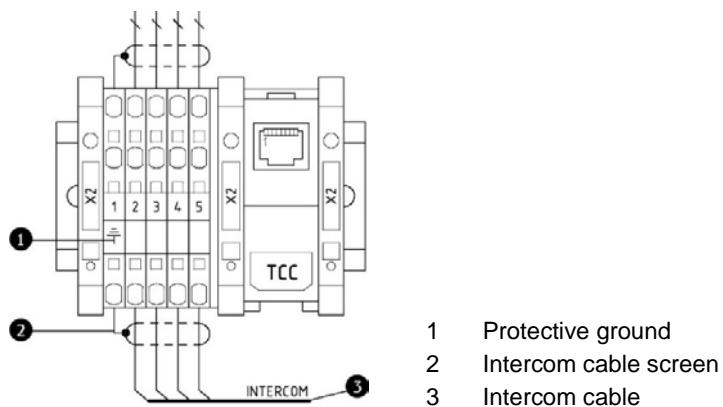
Fig. 37: Terminal block -X2, connection intercom system, with 4-wire connection
