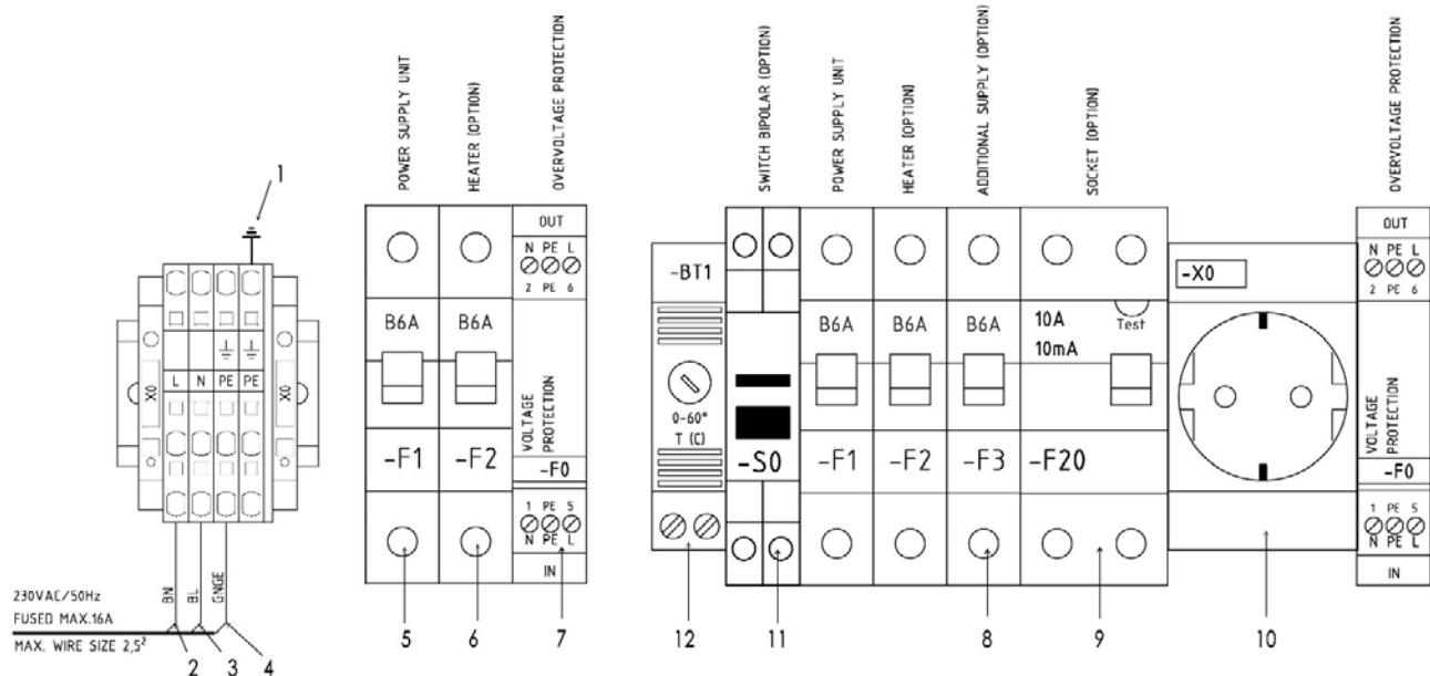
Fig. 32: Terminal block -X0, power distribution box (basic equipment and with optional components)
