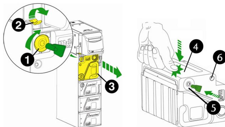
Fig. 90: Removing and opening the banknote cassette
