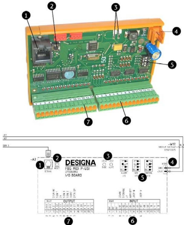
Fig. 44: I/O interface Midi-P-USI (here I/O interface assignment of an entrance control terminal)
