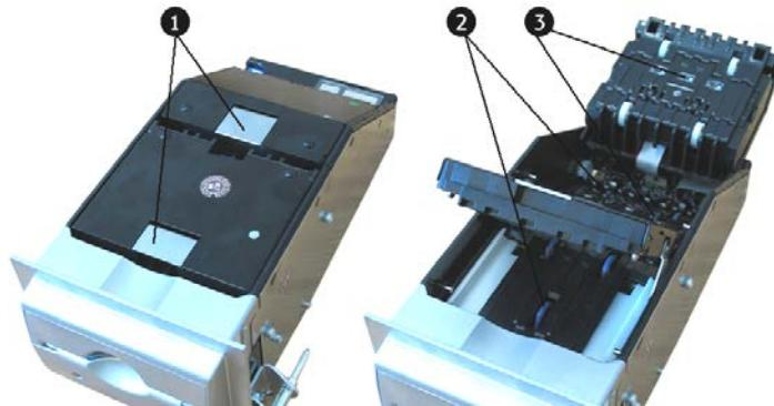
Fig. 78: Cleaning the banknote reader
