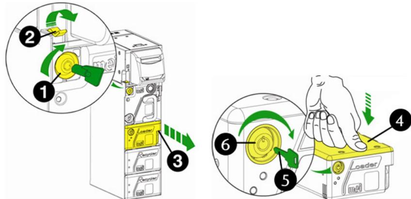
Fig. 91: Removing and opening the loader cassette
