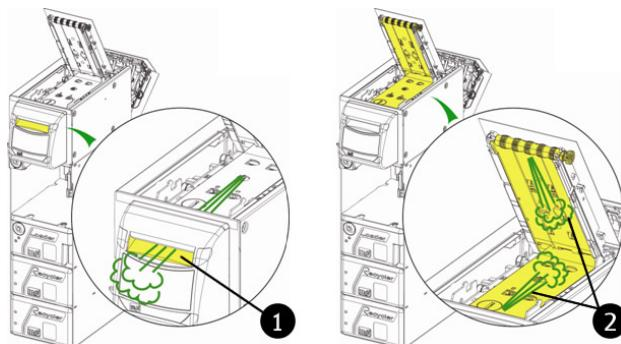
Fig. 97: Cleaning the banknote accepter and the positioner
