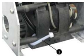
Fig. 48: Feeding channel I blocked
