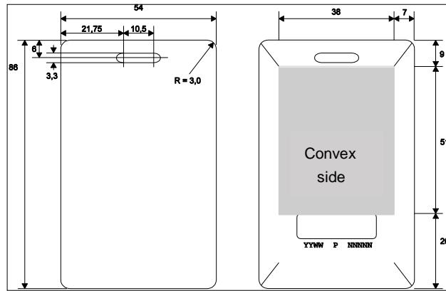
Fig. 106: EasyMove card (active): Approx. dimensions in mm
