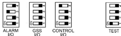
Fig. 45: DIP switch positions
