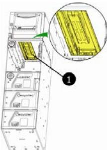
Fig. 102: Banknote cassette-pressure plate
