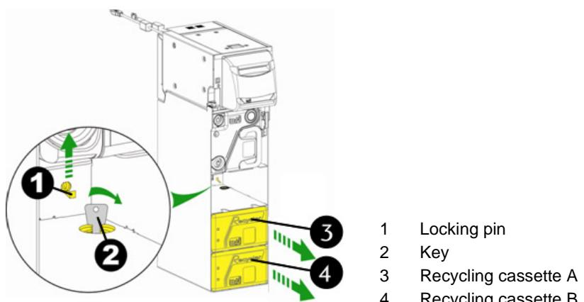
Fig. 103: Removing the recycling cassette
