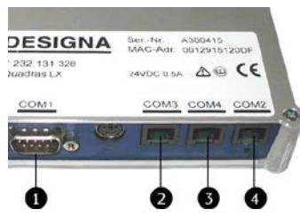
Fig. 41: Serial interfaces
