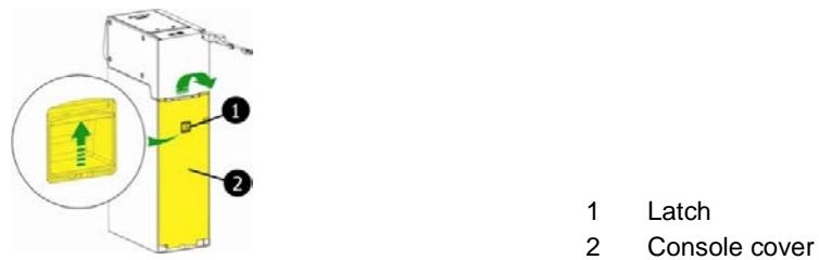
Fig. 99: Opening the console cover
