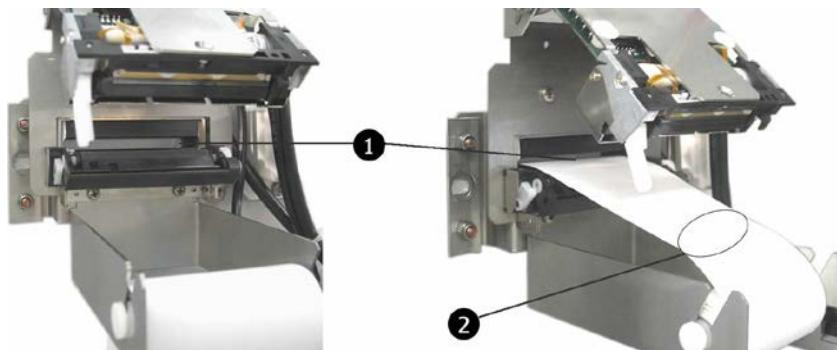
Fig. 73: Feeding paper into the draw-in device
