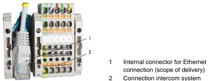
Fig. 11: Terminal block -X2 (similar to figure)
