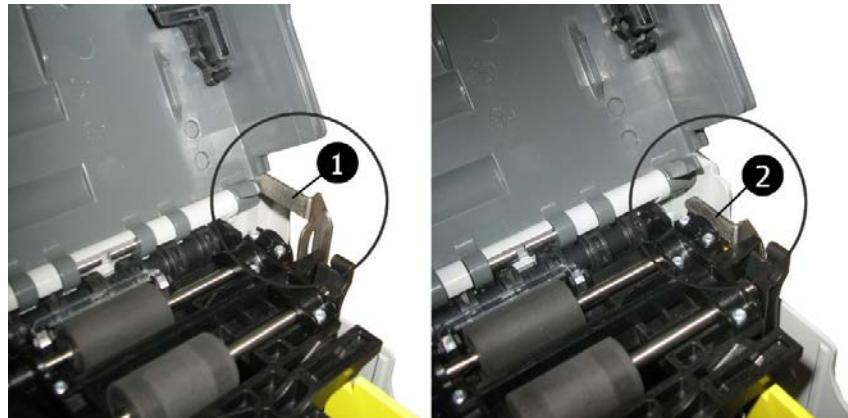
Fig. 92: Loader cassette, locking latch: correct position (left), wrong position (right)
