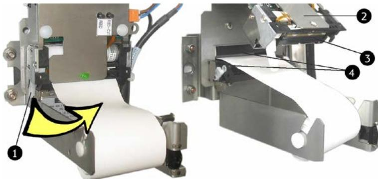
Fig. 74: Releasing the opening lever to loosen the print head from the paper reel
