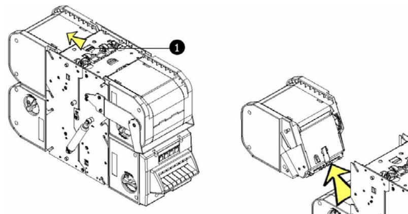
Fig. 83: Removing the recycling or (multi-)escrow cassettes
