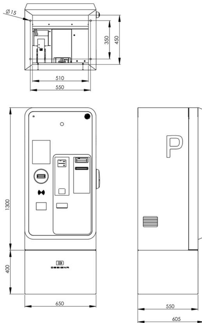
Fig. 5: Pay Coinless, with optional illuminated frame, dimensions in mm
