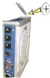
Fig. 43: Replacing the battery at the LCC
