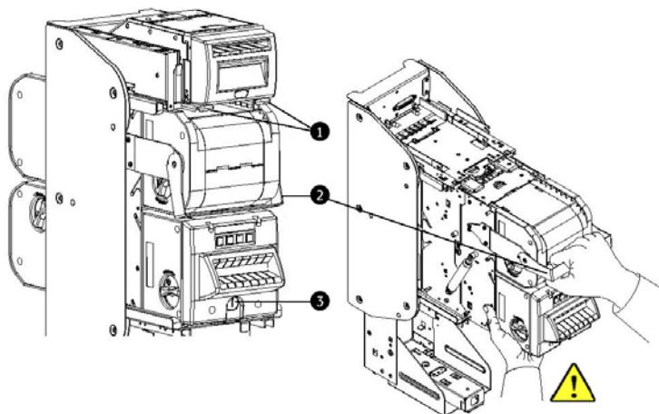
Fig. 79: Removing the chassis
