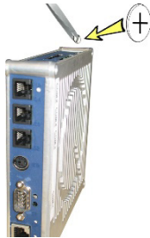
Fig. 39: Replacing the battery at the LCC
