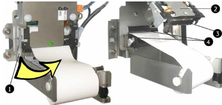
Fig. 31: Releasing the opening lever to loosen the print head from the paper reel
