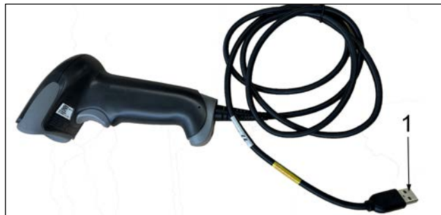
Fig. 13: Connection barcode / QR-code scanner (similar to figure)
