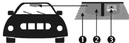
Fig. 54: Windscreen with a partial vacuum-metallized surface
