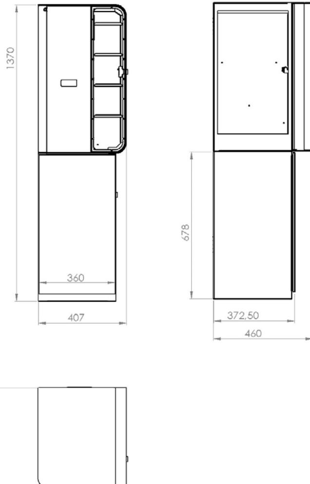
Abb. 4: IN/OUT, Abmessungen in mm
