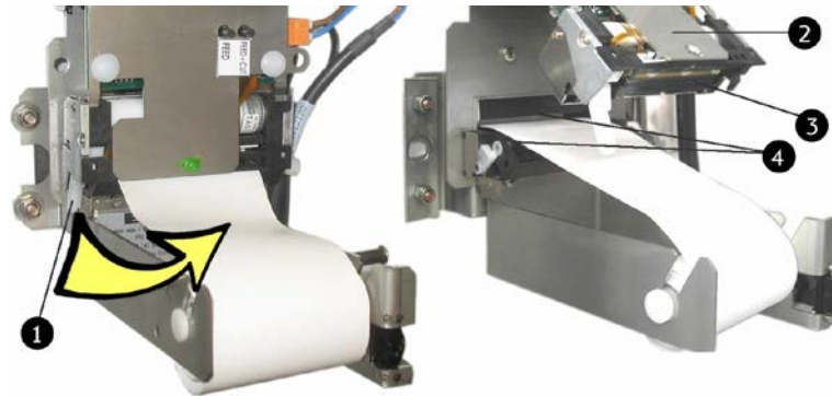
Fig. 78: Releasing the opening lever to loosen the print head from the paper reel
