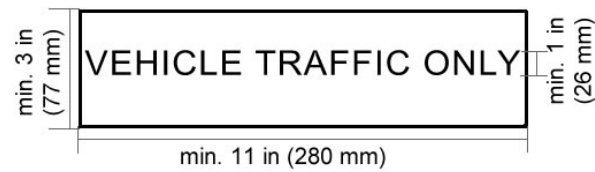
Fig. 3: Gate's danger zone sign II
