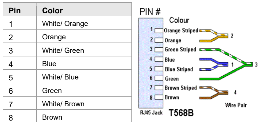
Fig. 37: Assignment of the Ethernet connection, EIA/TIA-T568B
